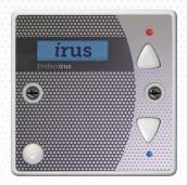
The concentration of  $\mathrm{CO}_2$  is determined by passing infrared light through a sample of the air and comparing absorbtion of light at two different wavelengths. The sensor combines this information with barometric pressure and temperature measurements to calculate  $\mathrm{CO}_2$  concentration.
