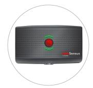
Check the condition of the case for cracks or damage and ensure there are no signs of tampering.
