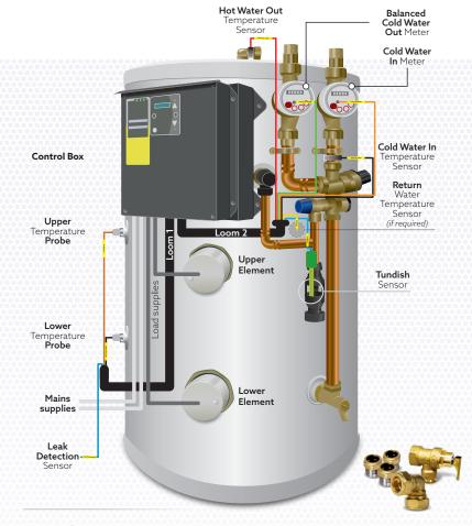
irus SMART Tank is an unvented stainless steel direct cylinder, factory fitted with Prefect Controls SMART Control Unit - Pre-wired and Pre-plumbed.
