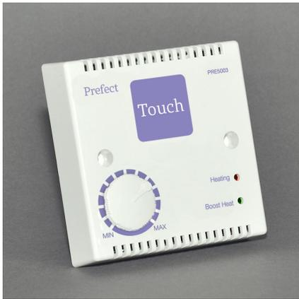
The Thermostat should be mounted at least 300mm away from the heater, and protected from artificial heat sources for example: Desktop computers, TV's, Desk lamps etc. The Thermostat should be mounted at chest height or mounted in the dado trunking above the workstation. Mount in a 25mm or greater back box.
