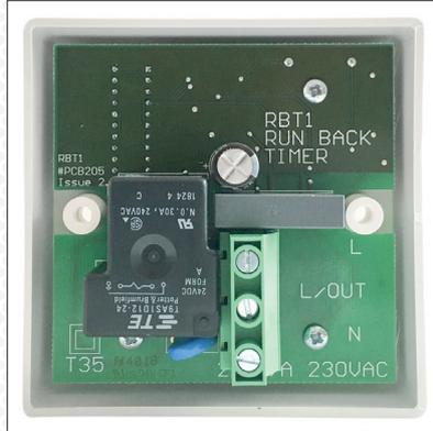
Mount in a surface or sunken pattress box of 25mm or greater. If fitting to a metal back box ensure that top and bottom lugs are removed.
