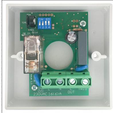
Mount in a surface or sunken pattress box of 25mm or larger. To switch from more than one position simply wire two or more units in parallel to achieve two way and intermediate switching, or use the trigger terminal with a slave switch.
