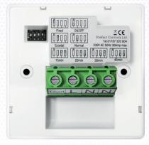
Two modes of operation are available: Fixed mode and ON/OFF mode. When set to fixed mode the time run will start on a button press and will continue until the time run has elapsed. When set to ON/OFF mode the time run can be stopped at any point during the time run.
